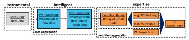
Figure 3 - Aggregation process from measuring data to condition indicator
