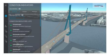
Figure 6 - Overview on the web-interface conditionCONTROL
